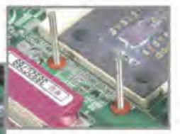
Place and tighten four nuts all the way down.
